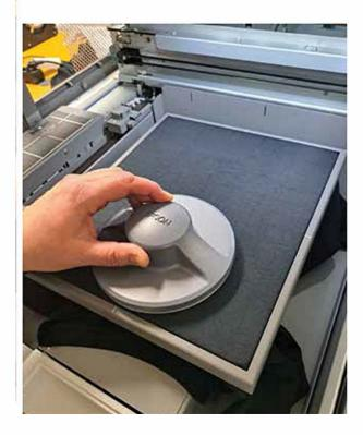
Notice that the image on printer display point the opposite side than the shirt on print bed. Start print by pressing "Start" button.
