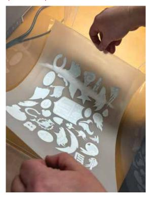
Place the film to Siser heat press (make sure the upper plate doesn't touch the powder) in 200°C about 10 minutes, until the melted powder looks like orange skin.
