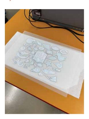
Place the film on the bottom of the plastic box and sprinkle the hot melt powder on the printed areas .
