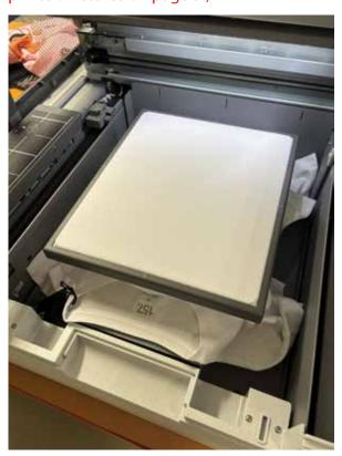
Level the surface of the fabric with this tool.
