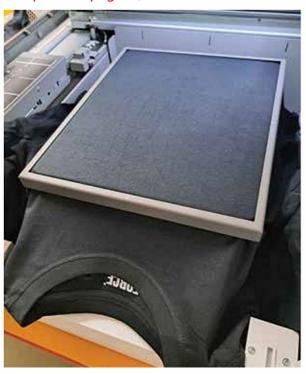
Wrap the shirt on top of the frame. Turn the package 180 degrees so that the neckline points downwards.
