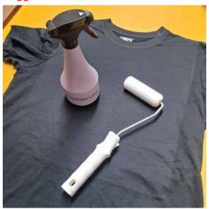
Try to use the same direction when spraying and don't overlap, the already sprayed areas too many times. This could lead to some areas being overly pre-treated and others having less pre-treatment, which would cause an uneven print with patches.
