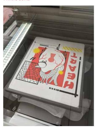
Heat press the image in 175°C for 90 seconds. REMEMBER to use baking paper to protect the image.
