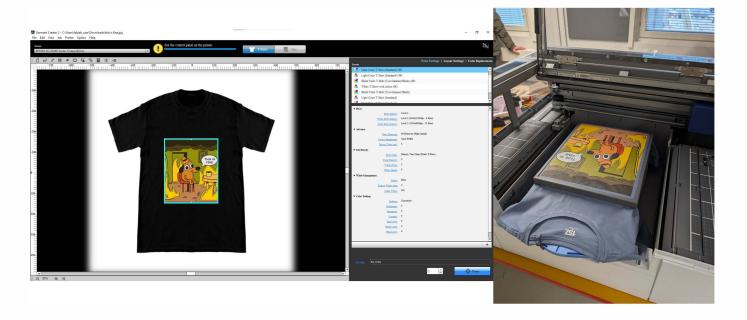
If youre printing a horizontal picture (image flipped 90 degrees counterclockwise), the shirt must be placed this way (notice where the neck is). This way its possible to use the whole print area for a horizontal print.
