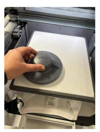
Notice that the image on printer display point the opposite side than the shirt on print bed. Start printing by pressing Start button.
