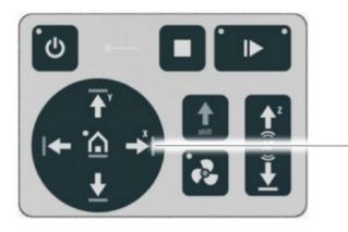
1. Use the X/Y position keys on the control panel to move the processing head over the material to be engraved.
