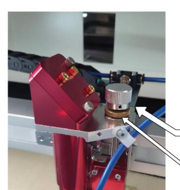
3. Turn down the processing head with the adjusting screw until the focus tool falls down.
