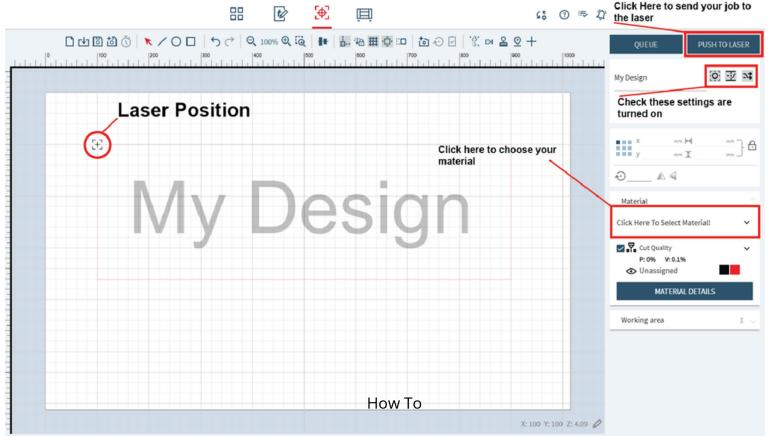
To prepare our job for the laser cutter first we have to position our job on the bed, to help us do this we can use the red laser positioning dot as a guide.
