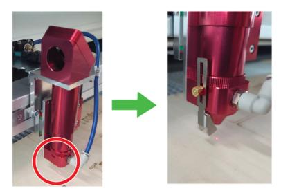
2. Place the focus tool on the processing head.
