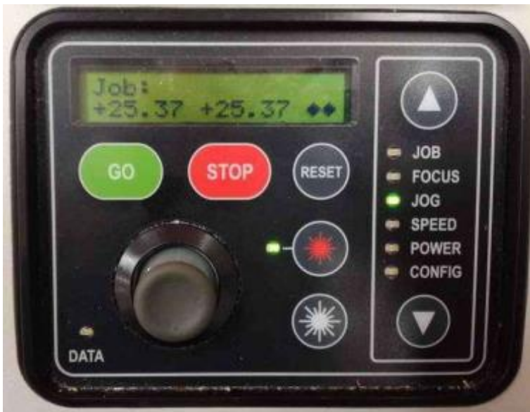
Fig 3: Control panel in JOG mode.
