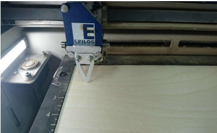
Fig 2: Focusing triangle at right height for 4 mm plywood
