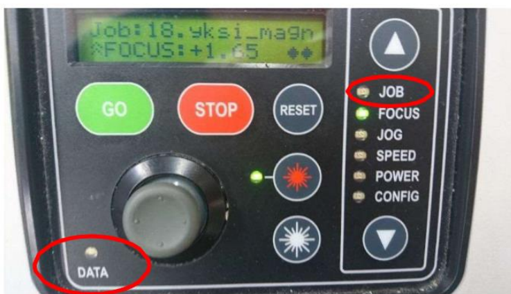
Fig 13: Choose Job from control panel and make sure that the Data light has stopped flashing.
