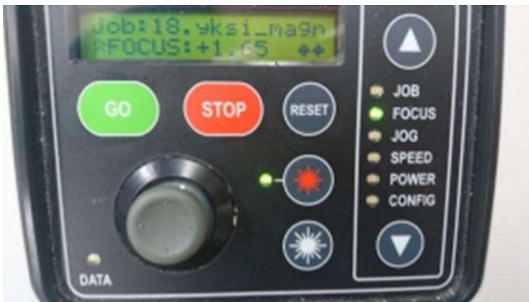
Fig 1: Control panel in focus mode
