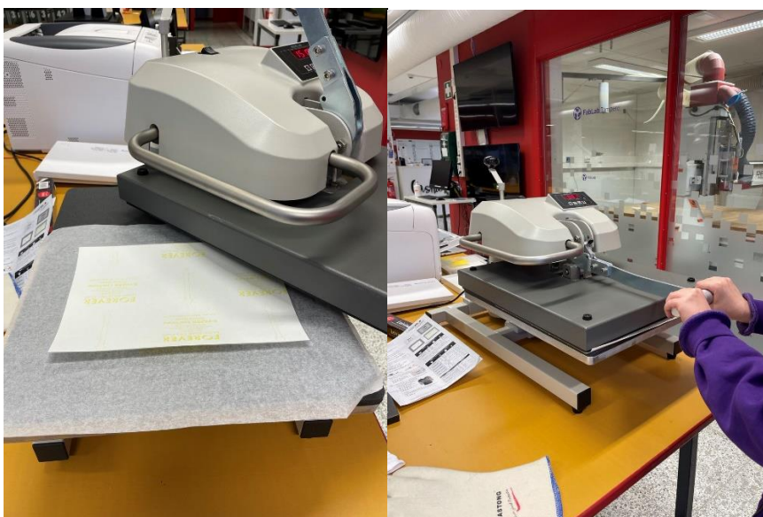
Figure 13: Setting for the first press. Lock the press down with the lever.
