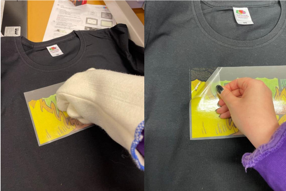
Figure 17: Rub the print thoroughly with a mitten. When the paper is ready for removal, remove it with smooth and low motion.
