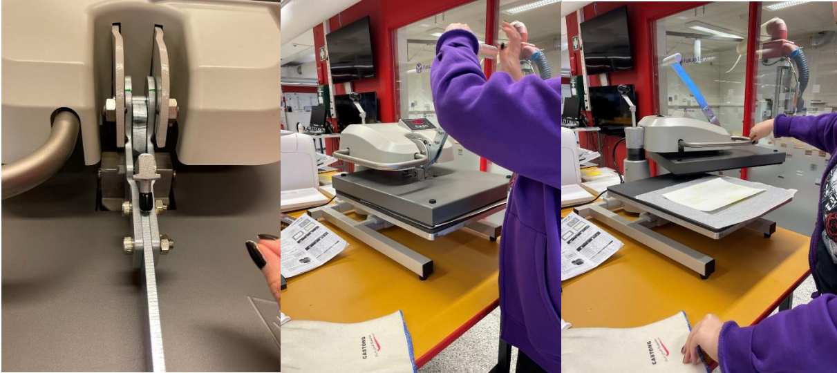
Figure 14: On the left: Remove the small certifier to this position to open the press. Open press by lifting the lever and sliding the top part to right.
