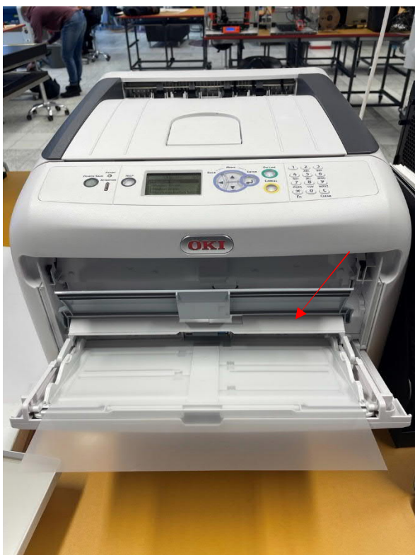
Figure 10: Put the foil printing side up by carefully lifting the lid.
