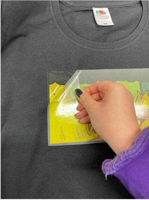
Figure 17: When the paper is ready for removal, remove it with smooth and low motion.
