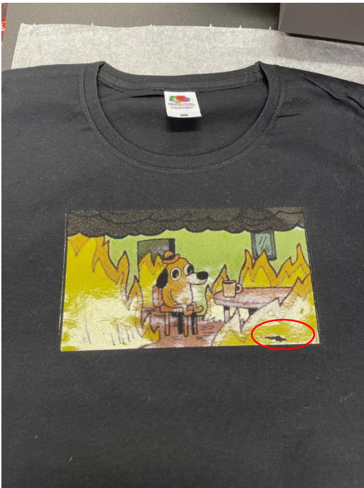
Figure 18: Freshly pressed image that has ripped slightly.
