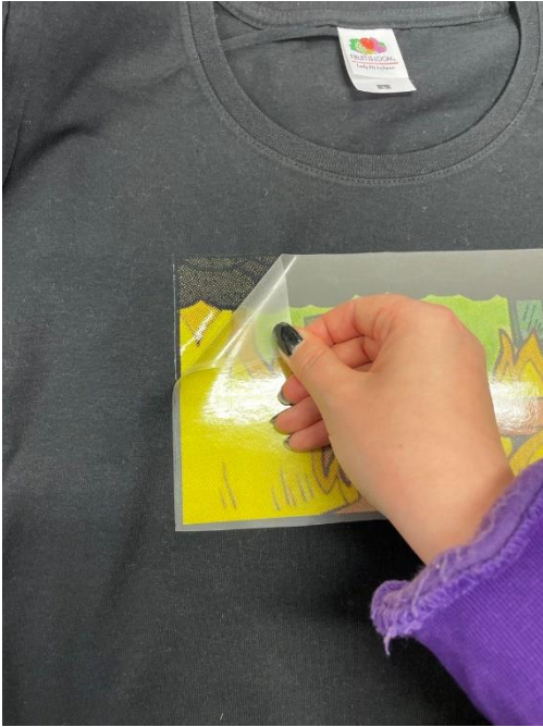
Figure 16: When the paper is ready for removal, remove it with smooth and low motion.
