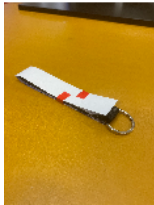
Key chain - actual size 22x125 mm (one side), print size 27x270 mm (both sides), heat press temp. 200 C°, time 40 sec.
