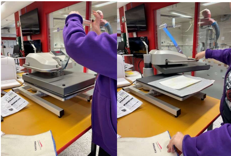
Figure 13: Open press by lifting the lever and sliding the top part to right.
