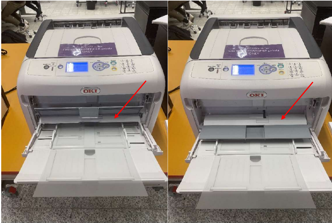
Figure 9: Put the foil printing side up by carefully lifting the lid.
