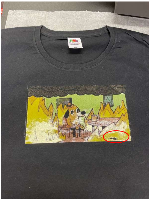
Figure 17: Freshly pressed image that has ripped slightly.
