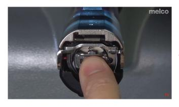
PUT YOUR THUMB ON THE THREAD AND INSERT THE BOBBIN CASE BACK TO THE MACHINE PRESS SO THAT YOU HEAR A CLICK.
