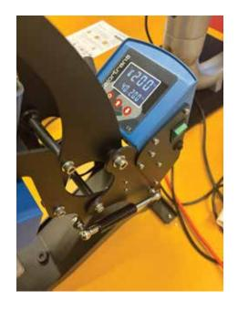
Turn on the heat press and set the temperature to 200 C° and time to 40 sec.
