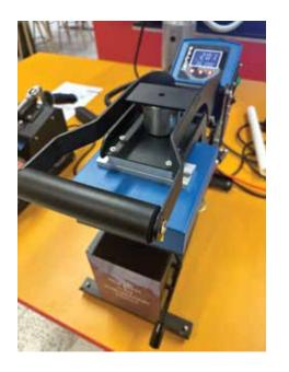
Turn the handle down until it locks. The clock starts to count down. After 40 seconds the handle opens up automatically.
