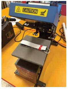
Place the key chain inside the heat press like this.
