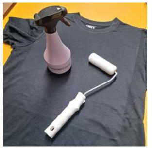
Try to use the same direction when spraying and don't overlap, the already sprayed areas too many times. This could lead to some areas being overly pre-treated and others having less pre-treatment, which would cause an uneven print with patches.
