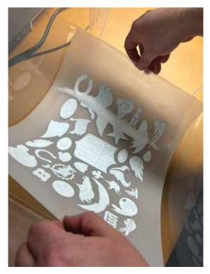
Place the film to Siser heat press (make sure the upper plate doesn't touch the powder) in 200C° about 5 minutes, until the melted powder looks like orange skin.
