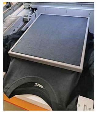
Wrap the shirt on top of the frame. Turn the package 180 degrees so that the neckline points downwards.
