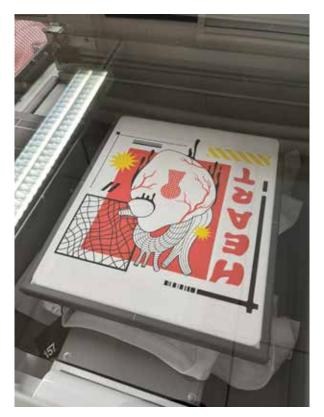
Heat press the image in 175C° for 45 seconds. REMEMBER to use baking paper to protect the image.
