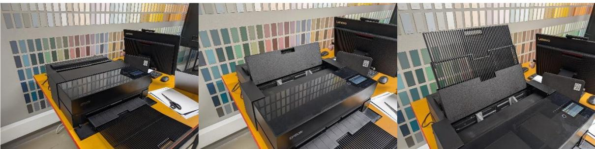
Feed one sheet of paper in portrait orientation, face up. Make sure the gray clips hold the edges of the paper.
