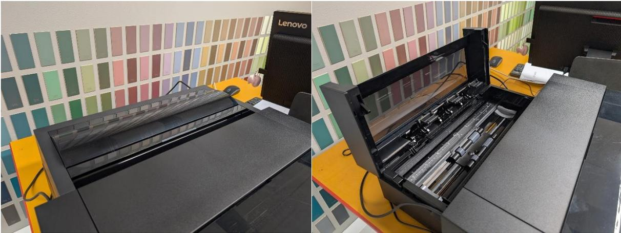
Place the roll you are using in the case so that the roll is unloaded from the top into the printer. Feed the paper until you hear a beep. Close the lid.
