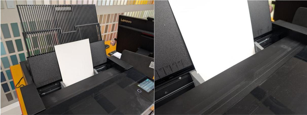
When the printer detects the paper, the rear paper feeder menu opens in the printer window.
