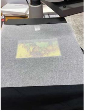
Pressing your image to the cotton fabric, temperature should be 150 °C and timer 30 seconds. Set the timer as you did before. Now you can do the pressing.
